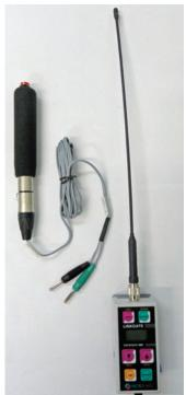
Special thanks go to The Southern Trust for making grant funds available for the purchase of a mobile starting transmitter. This is similar to the radio transmitter at the 2000m start but can be used from any point on the course to automatically trigger the control room timing and camera computers.
